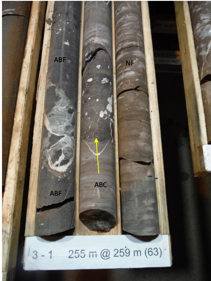
Fig.6 Amygdaloidal basalt flow (ABF) and clast (ABC) (two runs on left); interlayered with and passing down hole into fossiliferous/calcareous clastic sedimentary rocks and interlayered nodular limestone (NL) (run on right).
