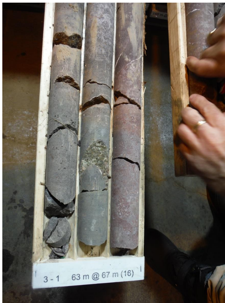
Fig 1. Massive green andesite (two runs on left) gradational down hole into red (oxidized), amygdaloidal andesite clast, interflow unit (run on right).
