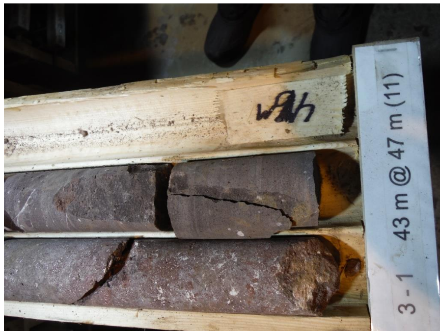
Fig. 3. Andesitic interflow fragmental unit (bottom run); on top of a massive to slightly amygdaloidal andesite flow (top run).
