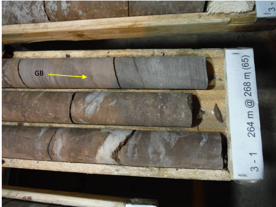
Fig 7. Calcareous sedimentary rocks (bottom two runs) interlayered with grit (top run). Note, graded grit beds (GB) with erosional lower contact clearly illustrating tops/younging direction up hole.
