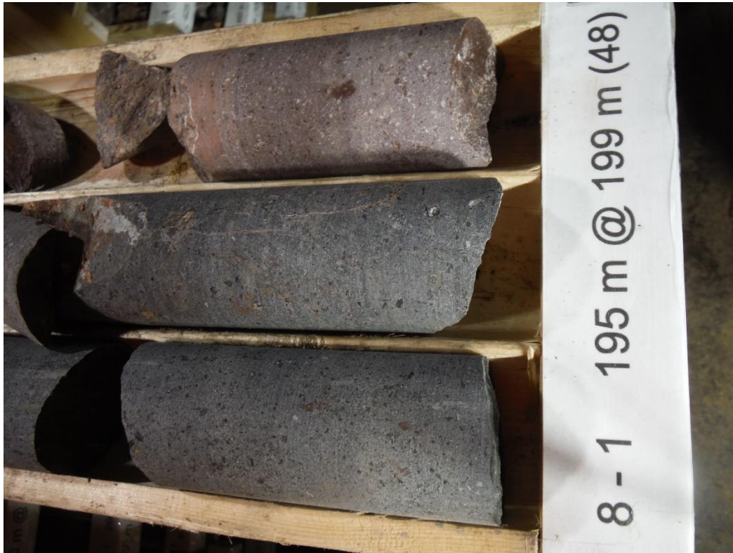
Fig. 11 Maroon to green-grey crystal lithic tuff (andesite) from drill core 8-1 at 195-199m m.
